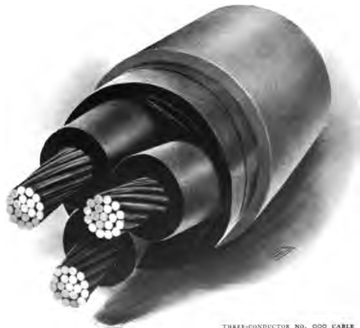
THREE-CONDUCTOR NO. 000 CABLE FOR 11,000 VOLT DISTRIBUTION
